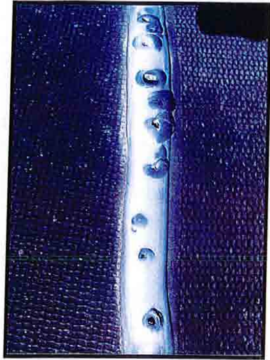
Typical "Bubbling" Failure of Extrusion Weld
