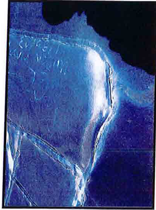
Typical Peel Failure of Extrusion Weld
